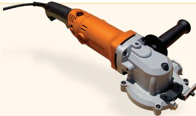
**BNCE-20 The Original Cutting Edge Saw™** A multipurpose cutting tool. It can easily cut #6 (3/4") rebar, all-thread rod, chain, EMT conduit, copper pipe, steel rods, steel tubing, and much more. This AC powered hand-held tool is lightweight and features a three position handle. The capacity of the opening is .875" (23.62mm). This tool is ETL Listed and is excellent for cutting rebar or bolts near flush with concrete or block construction.
