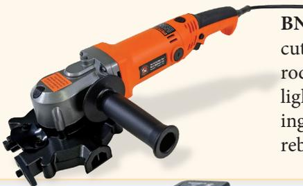
**BNCE-30 Cutting Edge Saw™** A multipurpose cutting tool. It can easily cut #8 (1") rebar, all-thread rod, chain, EMT conduit, copper pipe, steel rods, steel tubing, and much more. This AC powered hand-held tool is lightweight and features a three position handle. The capacity of the opening is 1.18" (30mm). This tool is ETL Listed and is excellent for cutting rebar near flush with concrete or block construction.
