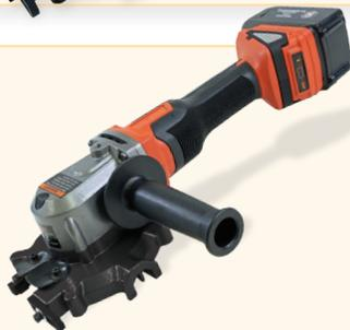
**BNCE-30-24V Cutting Edge Saw™** This is a 24V battery-operated multipurpose cutting tool. Like the corded model above, it can easily cut #8 (1") rebar, all-thread rod, chain, EMT conduit, copper pipe, steel rods, steel tubing, and much more. It also features a three position handle. The capacity of the opening is 1.18" (30mm). This tool comes complete with two (2) Li-Ion Batteries and a charger.
