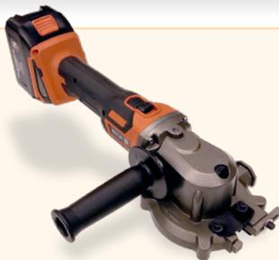
**BNCE-20-24V Cutting Edge Saw™** This is a 24V battery-operated multipurpose cutting tool. Like the corded model above, it can easily cut #6 (3/4") rebar, all-thread rod, chain, EMT conduit, copper pipe, steel rods, steel tubing, and much more. It also features a three position handle. The capacity of the opening is .875" (23.62mm). This tool comes complete with two (2) Li-Ion batteries and charger.
