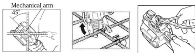
Unlock the trigger lock. Keep the mechanical arm on the rebars to be tied with a 45° angle at a vertical position to the rebars.
