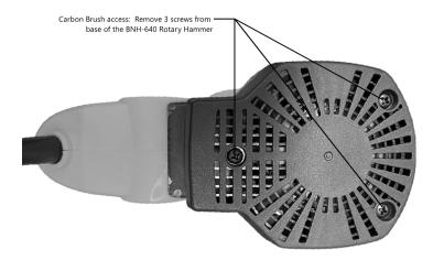
To re-install the brushes or replace with a new set, the brush should be inserted into the brush carrier subassembly, the lead wire connected, and the spring clip (coil spring) should be repositioned to firmly hold the brush into place. The wire lead must be reconnected to the wire lead connector.
