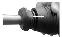
Slide the front of the chuck toward the body of the tool to insert, lock, and release an SDS Max bit
