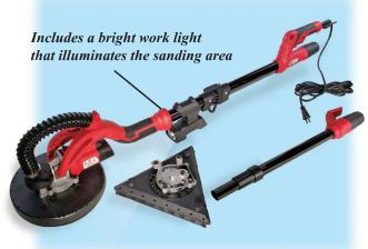
provide a large area of dust collection. The tool provides an easy hook-up with a standard vacuum hose to ensure a dust free working environment. With extension, you can easily reach up to 12 ft. The sanding head can be changed between a round head and a triangle head. The triangle head oscillates vs. the round rotating head. The triangle head allows for easier sanding along an edge of a wall or into tight spaces.
