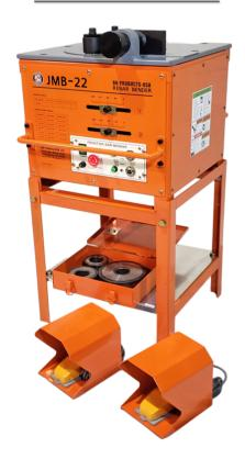
The **JMB-22 #7 Rebar Bender** is an electrical-mechanical bender, designed to bend up to #7 (7/8" or 22mm), Grade 60 rebar, up to 180° in *just 9 seconds*. This machine uses a 115V 50/60Hz 15 amp power supply, compatible with standard power sources.
