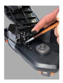
3. Hold the brake lever (reel press A) out while applying grease to the upper and lower points on the plunger (reel press axis). Some lubrication on the center axis is helpful. Spray lubrication is not reommended. If used, it should only be done sparingly because it can penetrate the case and get into the internal electronics of the tool.
