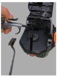
2. Clean the brake housing with compressed air or a brush
