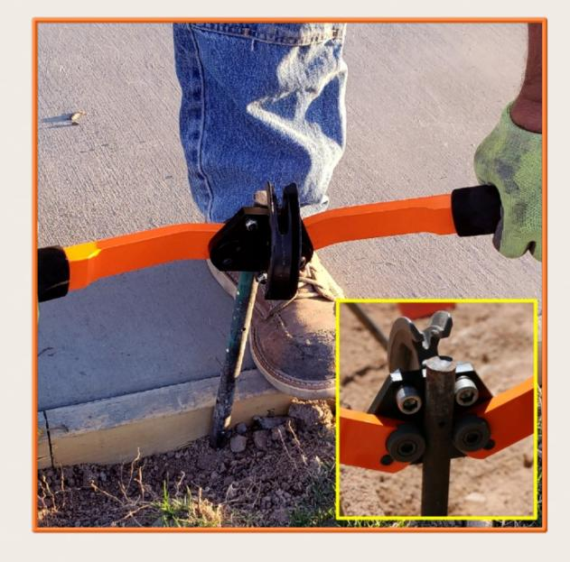
Align the Stake Puller around the stake, centered between the roller grips, with the rollers facing you.
