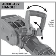
The auxiliary handle may be adjusted into any position around the shaft of the demolition hammer. To adjust the auxiliary handle, turn the handle adjustment knob counter-clockwise to loosen the handle.
