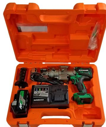
*The DCC-1636BHL Cordless Rebar Cutter* will safely and cleanly cut rebar up to 5/8" diameter; Grade 60. This self-contained electric/hydraulic unit will also cut other items like chain, bolts, and rod for use in multiple applications, including rescue operations. The cutting head quickly rotates up to 345° for use in vertical, horizontal, or difficult applications. A safety relief valve for retracting the piston and a cutting guard are standard features.
